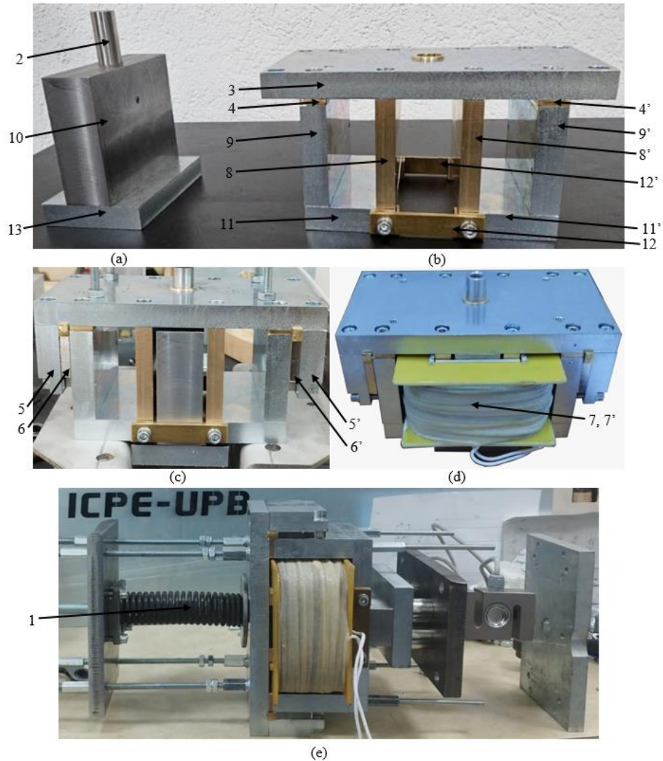
Fig. 7.6. Experimental implementation of the electromagnetic actuator model with permanent magnets; (a) – mobile ferromagnetic circuit; (b) – fixed ferromagnetic circuit; (c) – assembled ferromagnetic circuits; (d) – electromagnetic actuator assembly with permanent magnets, without opening mechanism; (e) – electromagnetic actuator assembly with permanent magnets, with opening mechanism
