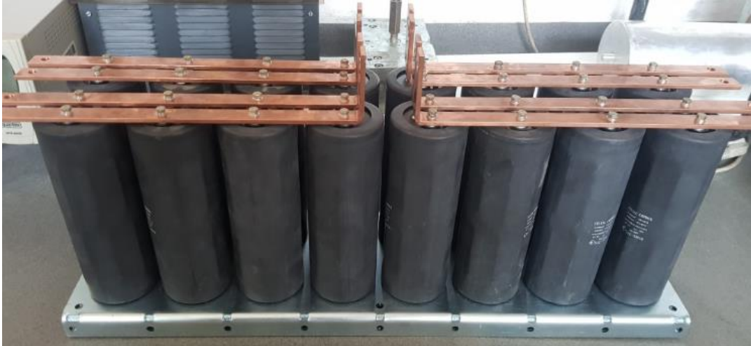
Fig. 8.1. Capacitor modules of the power supply for the electromagnetic actuator with permanent magnets
